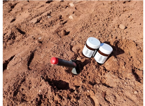
Figure 23. Sampling of remaining soil at the bottom of the excavation
