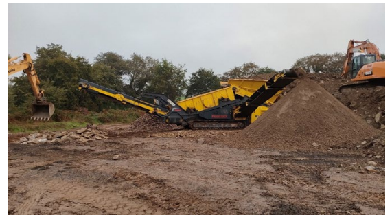
Figure 33. Screening of material for separation by size
