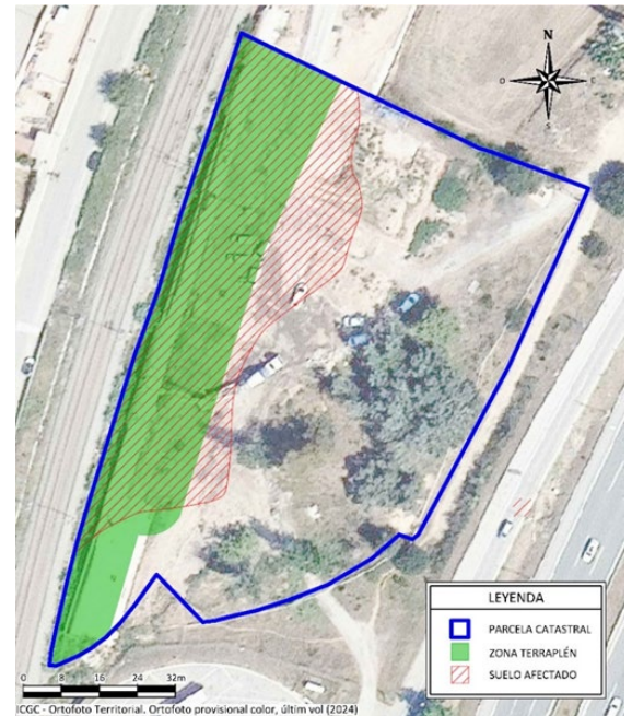
Figure 26. Material to be excavated for stockpiling
